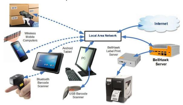
These BellHawk Servers are intended to be plugged into a site's local area network and to track manufacturing and warehousing operations at that site. With appropriate setup, however, users outside the site can still access the server over the Internet to remotely capture and view data, thus giving the best of both worlds.
