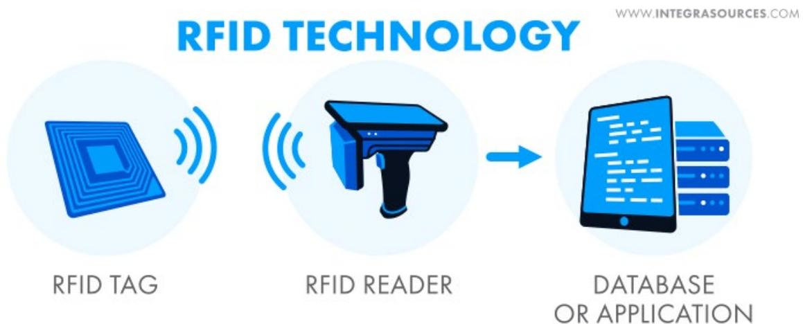
*ALT: A scheme showing an RFID reader receiving information from an RFID tag and transmitting it to a database or an application.*
