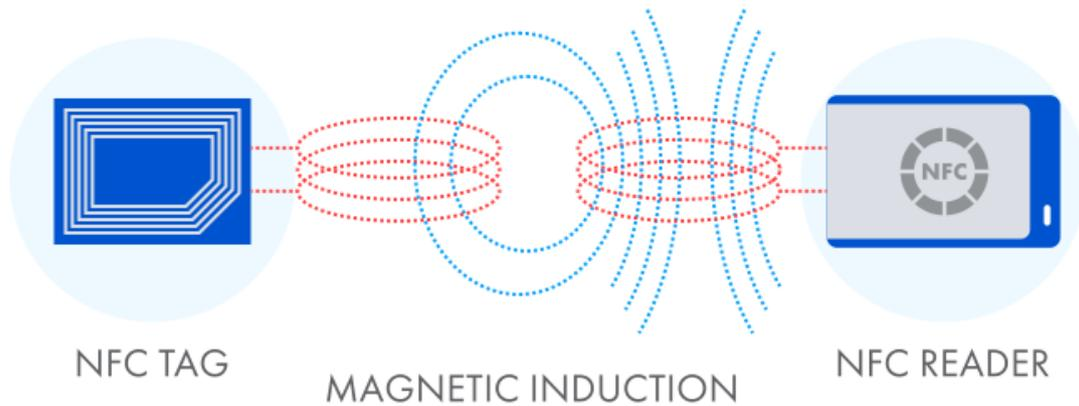
ALT: A drawing showing how NFC readers and NFC tags interact through magnetic induction.
