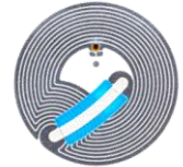
Eco friendly tags Paper based substrate and non-etched antennas
