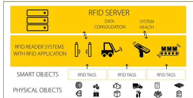
An RFID tag becomes energized when a radio signal from a 'reader' device triggers it, prompting the tag to transmit information encoded within it. RFID tags can store significant amounts of data, whether to identify a single component, or store installation information, manufacturing dates, or unique serial numbers.
