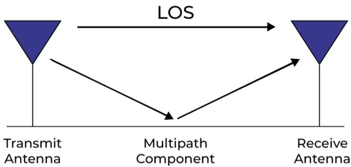
**Figure 7:** multipath interference diagram
