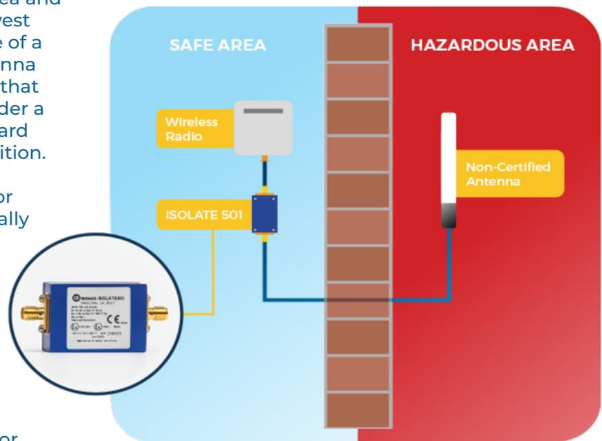
Figure 2: Typical safe area installation
