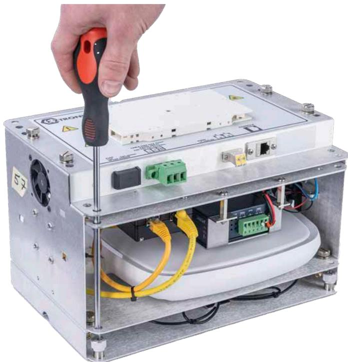
iWAP modular chassis system example with AP installed.
