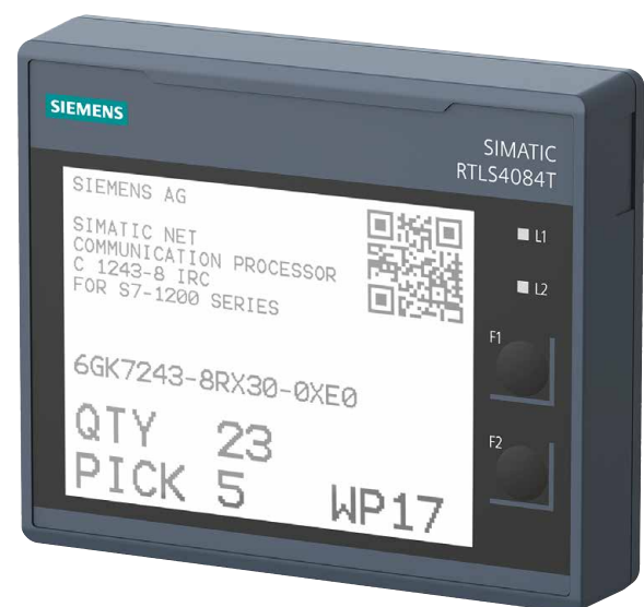
The ePaper transponder displays relevant information for production and logistics.
