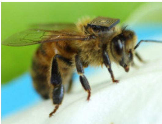
The bees manage to fly normally with the chip positioned close to their center of mass.
